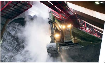
The bottom ash is washed with additional water in the slag extraction unit to reduce the content of readily soluble salts. It is sifted, broken up and freed from unburned components in order to produce a tested and approved building material comparable to a mineral mixture made from processed building rubble. The unburned components of the bottom ash are returned to the waste bunker to pass through the incineration process once more.
